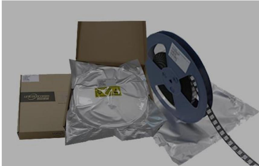
Figure 7-1 Module Package
